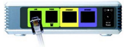
Figure 4-1: Connect to the Telephone Wall Jack
