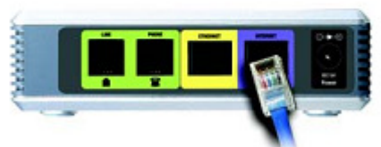
Figure 4-4: Connect to the Modem
